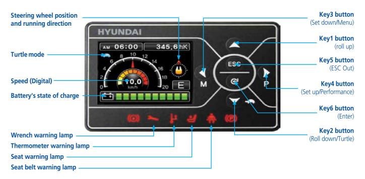
The LCD color monitor with 3.5 inch graphic smart display allows the operator to easily and efficiently control the machine. The monitor provides information about speed & accelerator level, steer angle & travel direction, battery discharge indicator, hour meter & working mode. The operator can select various performance modes to meet all working conditions. It is available multi-languages (maximum 11) for operator.
